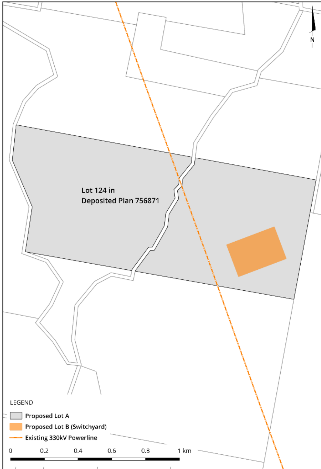
Figure 3-13: Subdivision Grid Connection Switchyard Lot 124
