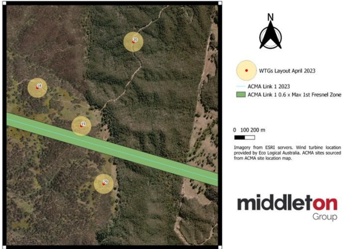
Figure 6-8: Location of Telecommunication Link Traversing the Project Site
