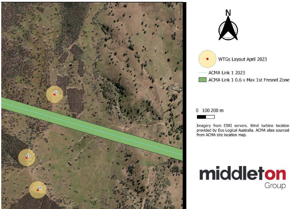
Figure 6-32: WTG 62 envelope based on 180 m rotor diameter, relative to the 0.6 threshold of the 1 st Fresnel Zone extent of the ACMA Link (Middleton, 2023)
