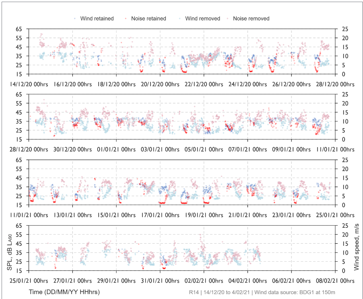
Figure 15: Receiver R14-1 background noise level and wind speed time history
