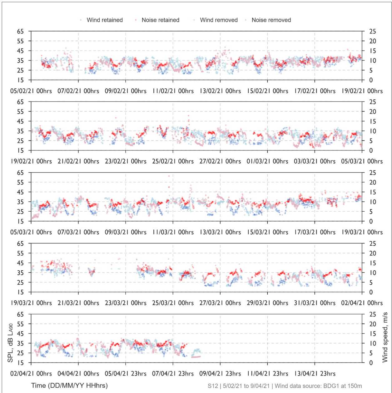
Figure 18: Receiver S12-1 background noise level and wind speed time history
