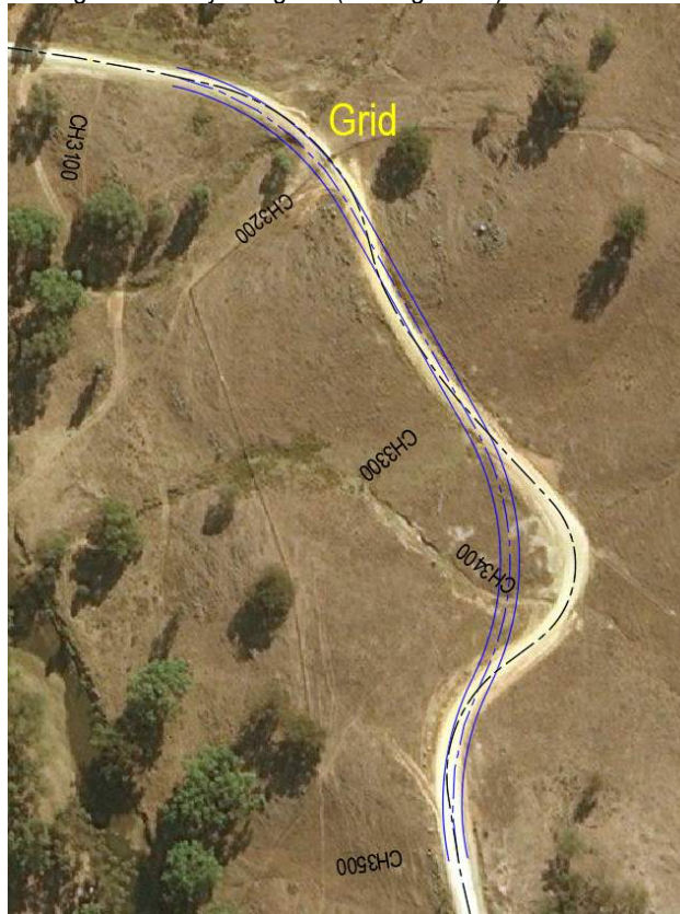
Figure 52 – Yarrabin Rd (CH 3,100 – 3,500), possible realignment
