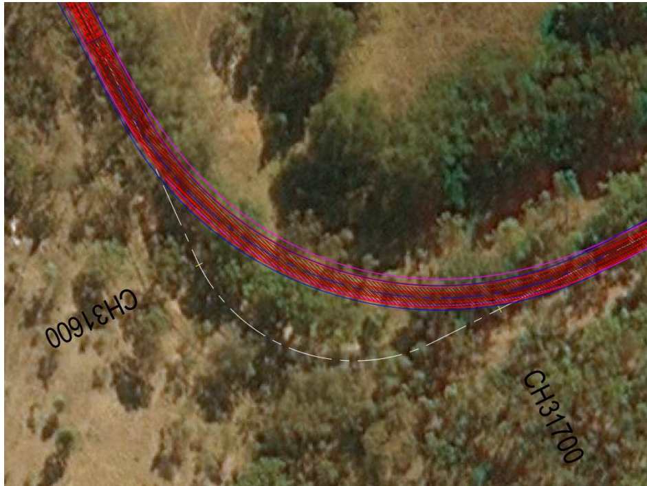
Figure 14 – Yarrabin Road CH 31,650 tight bend
