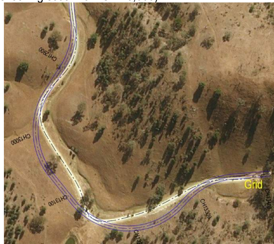
Figure 67 – Yarrabin Rd (CH 12,800 – 13,400), possible realignment
