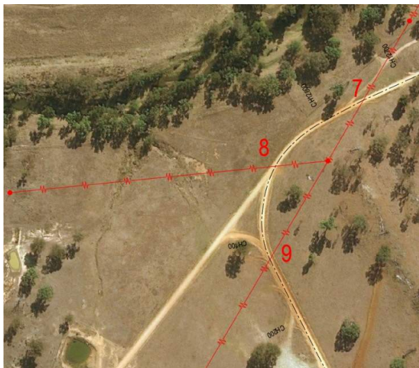
Figure B6 – Twelve Mile and Yarrabin Rd, Overhead Crossings
