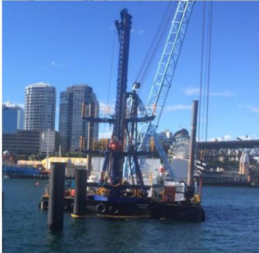
Crane Barge – new '35 Tonner' 32 m steel barge with slewing pin jib mounted crane
