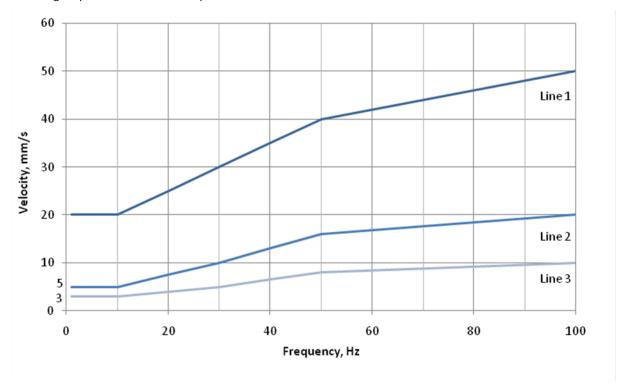
Figure 4.2 DIN4150 structural (cosmetic) damage guideline values of vibration velocity
