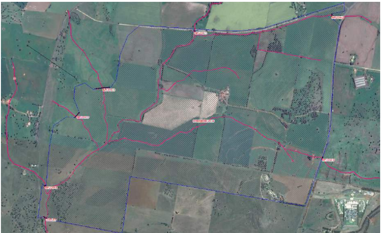
Figure 7: Two-Dimensional Flow Area and Hydraulic Boundary Conditions
