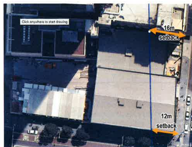
Figure 10 | Sightline (blue) and setbacks (orange) that would be required to retain views to Sydney Tower from Victoria Tower (source: DPE and Nearmap)
