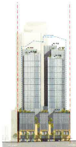
Figure 2 | Southern elevation of indicative mixed-use scheme with building envelope outline (blue hatched line) (Source: RtS).
