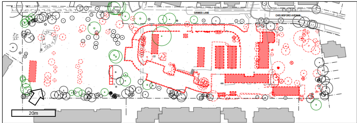
Figure 10 | Demolition plan (Source: Applicant's EIS 2021)
