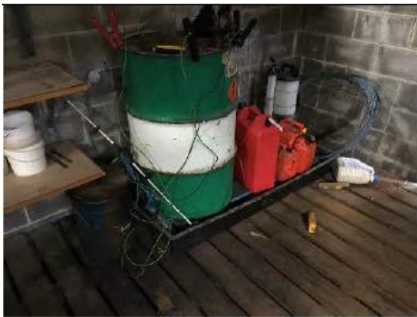
Photo 11 – Appropriate bunding for fuel storage.
