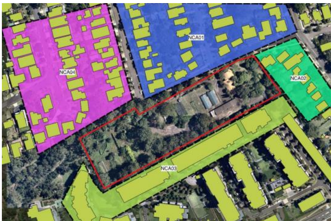
Figure 45 Noise Catchment Areas (Source: RWDI)
