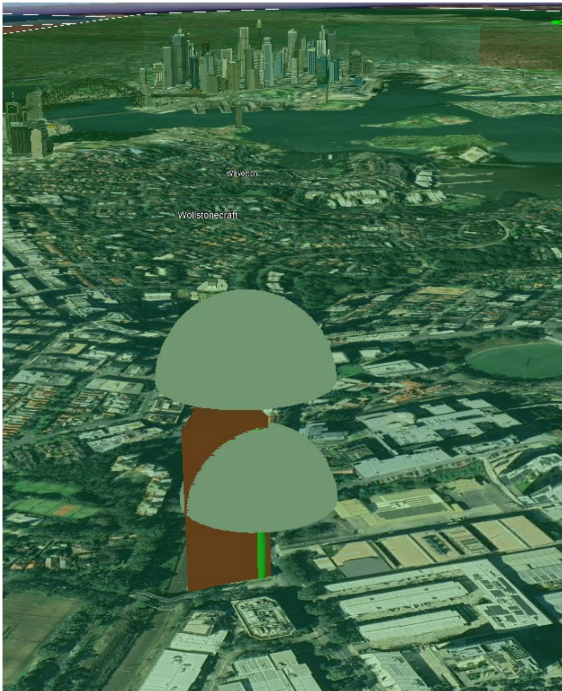
Figure 15: Avlaw's model of the proposed building and two (2) tower luffing cranes below the RTCC
