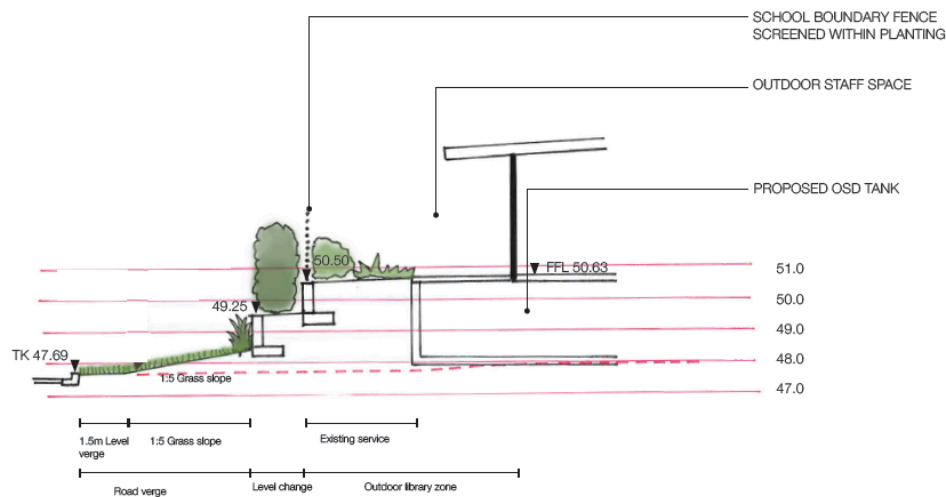
Figure 7-7 Section detail showing retaining walls on western boundary Source: Group GSA
