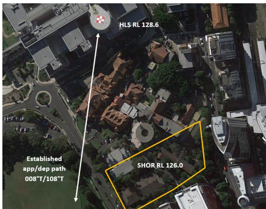
Figure 1: Site diagram of the planned SHOR construction and the main approach/departure flight path.
