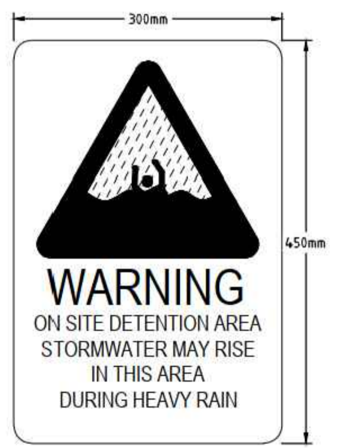
ON SITE STORMWATER DETENTION WARNING SIGN
