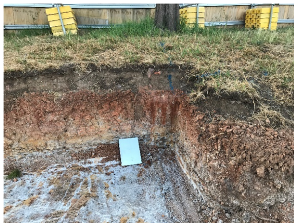
Photograph 1 : Subsurface soil profile exposed by excavation in the northeast corner of the site. The soil layers shown from top to bottom are:
