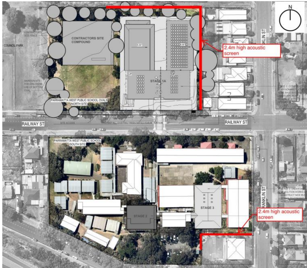
Figure 33: Extract from acoustic assessment showing screens during construction
