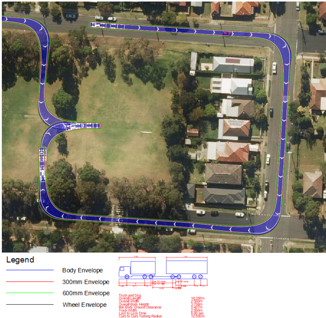
Figure A5: Swept path of 18.3 metre truck and dog entering the site from Crimea Street
