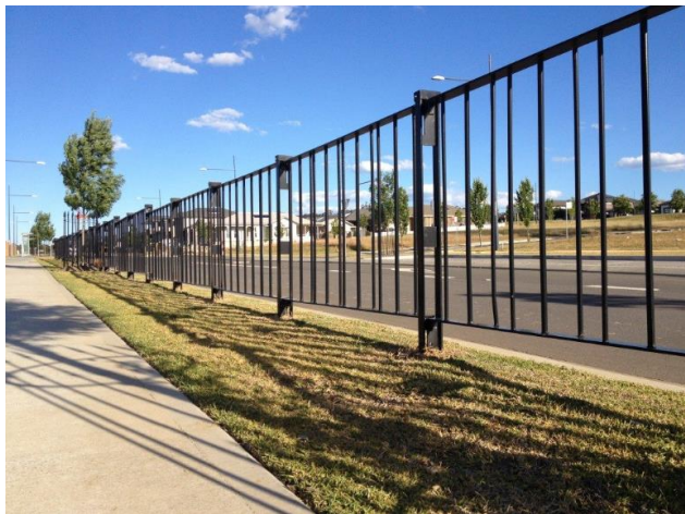
Figure 39: Typical RMS roadside fencing
