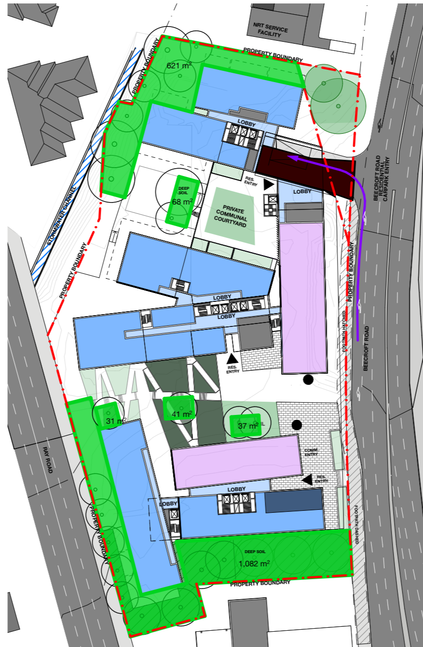
Image: Section 4.03 ADG - Deep Soil. Amended and approved Design Report, 19.03.20, Bennett and Trimble.
