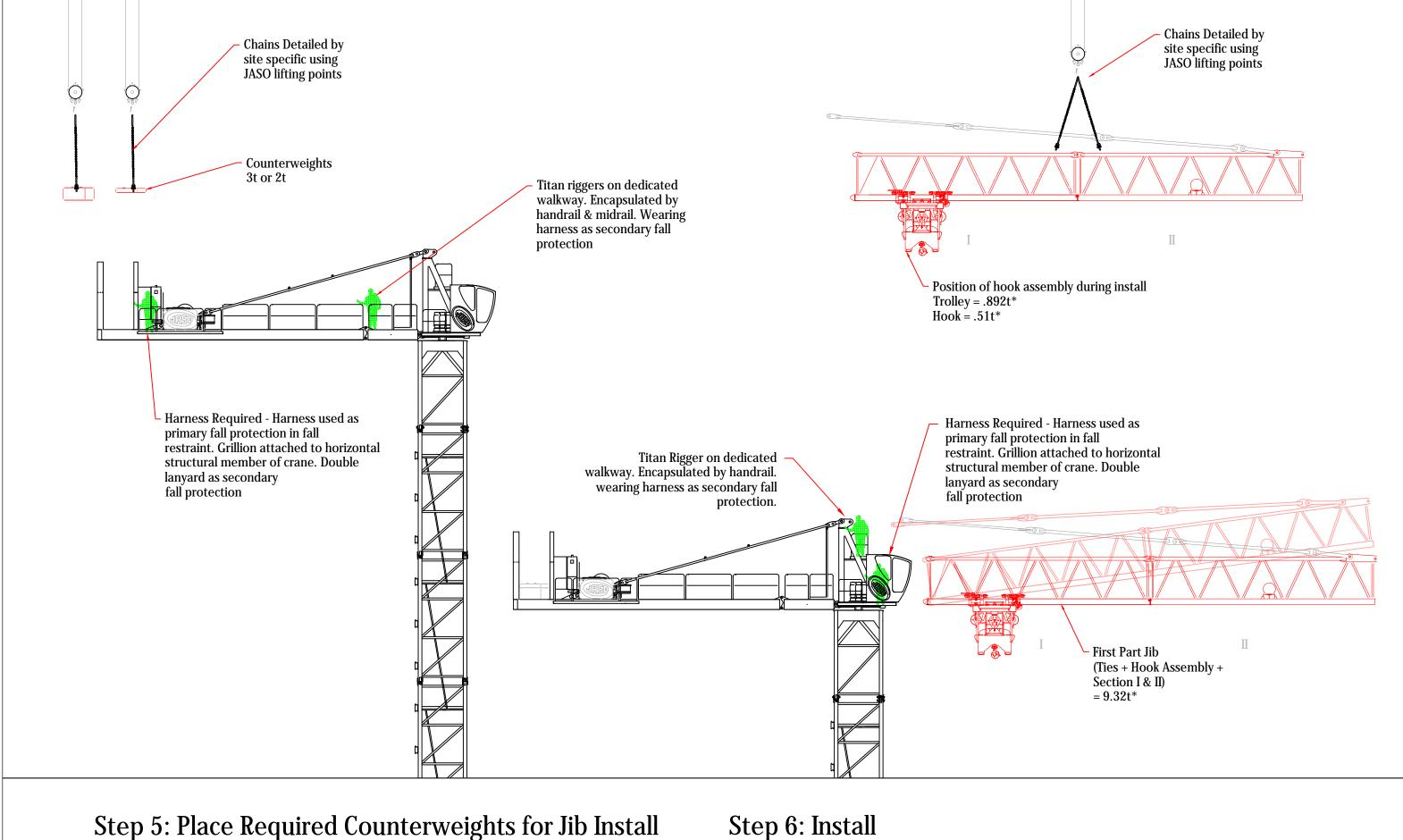
Step 5: Place Required Counterweights for Jib Install
