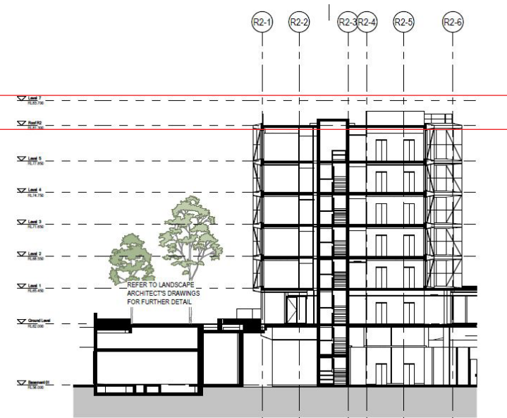
Above: Revised Design showing 3.1m reduction in height
