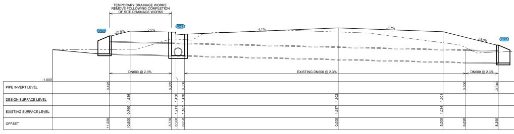
DRAINAGE PROFILE LINE 1 (AT CONTROL LINE CH 110.451) Scale Horizontal 1:50 Vertical 1:50
