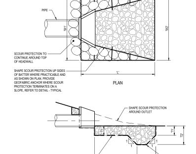
ROCKS TO BE PLACED OVER BIDIM A34 -GEOFABRIC OR APPROVED EQUIVALENT
