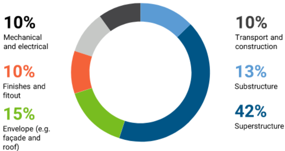
Figure 9: Typical breakdown of construction upfront carbon in a new office building (Source GBCA)
