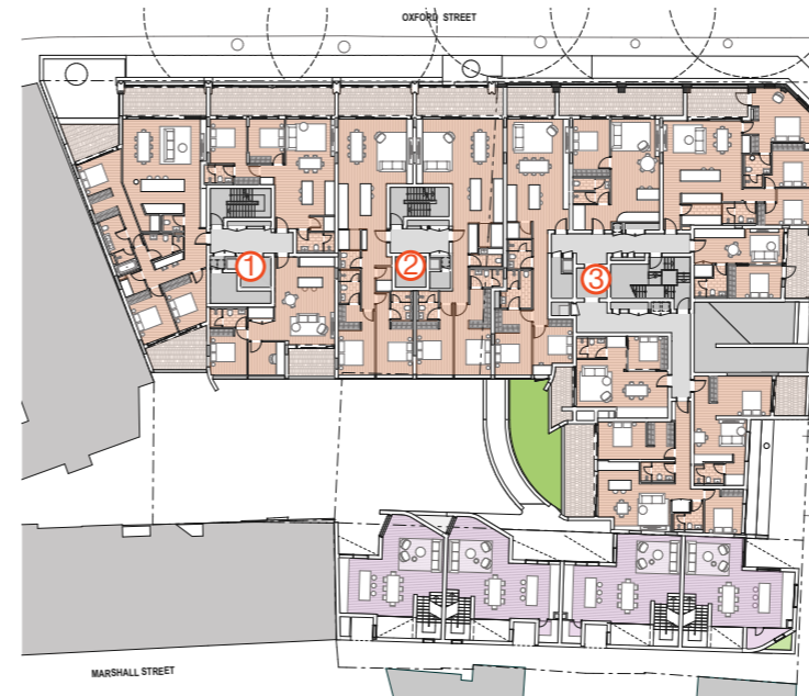
1. Typical Apartment Level, access from residential lifts 1, 2 and 3.
