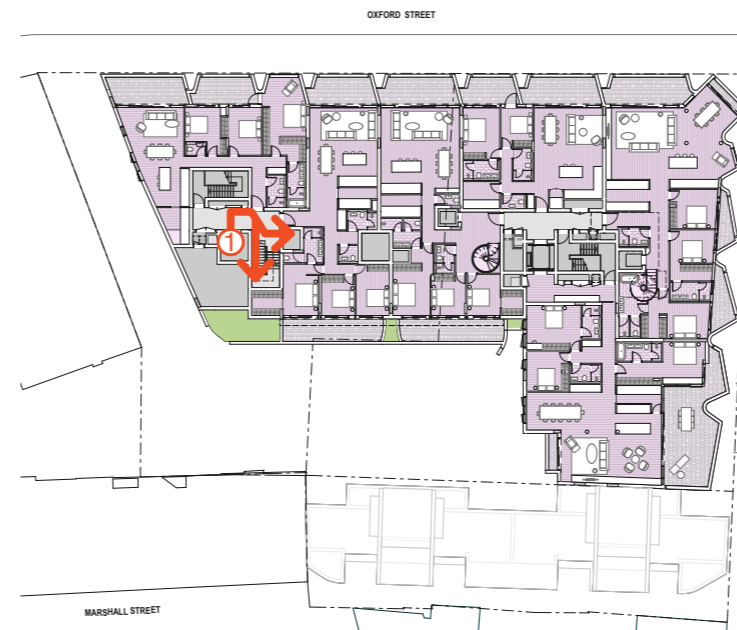
3. Lift 1 provides access from Ground to Level 6, where users transfer to either stairs or a secondary lift which takes them to Level 7.
