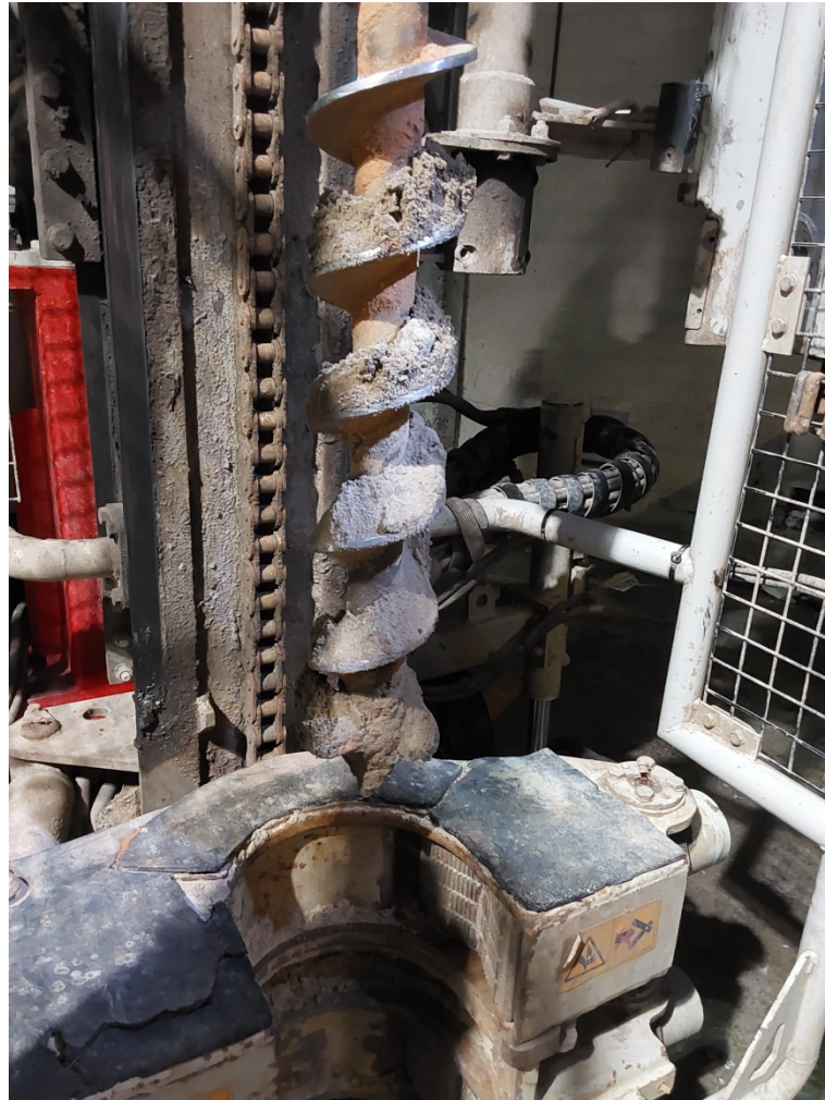
Photograph 3: Sandy Fill Material in BH103 (28/07/2023).
