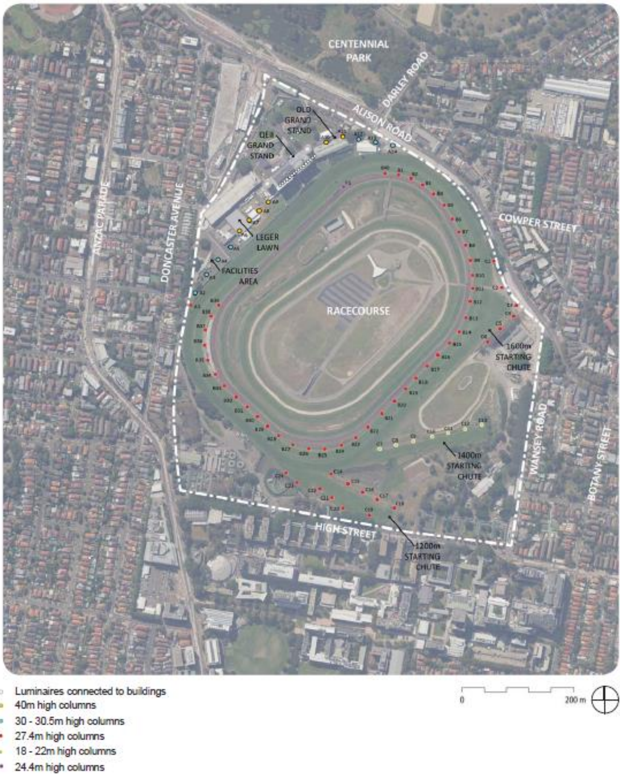
Figure 20 – Trackside Lighting Design – Heights of light columns
