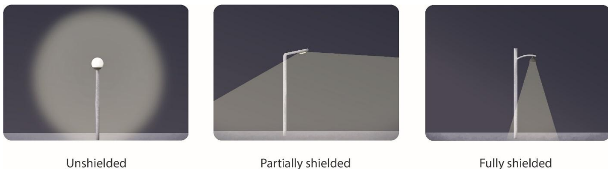
Figure 6-42 Light shielding (DCCEEW, 2020)
