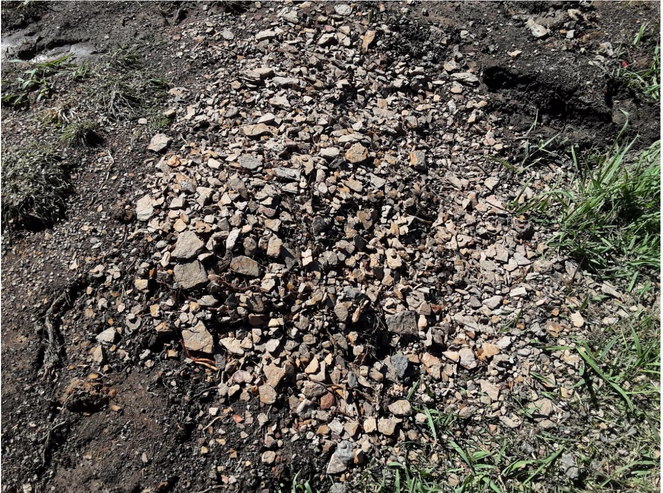
Photo 29 Remnants of sieving activities showing the extent of shale inclusions and stone material
