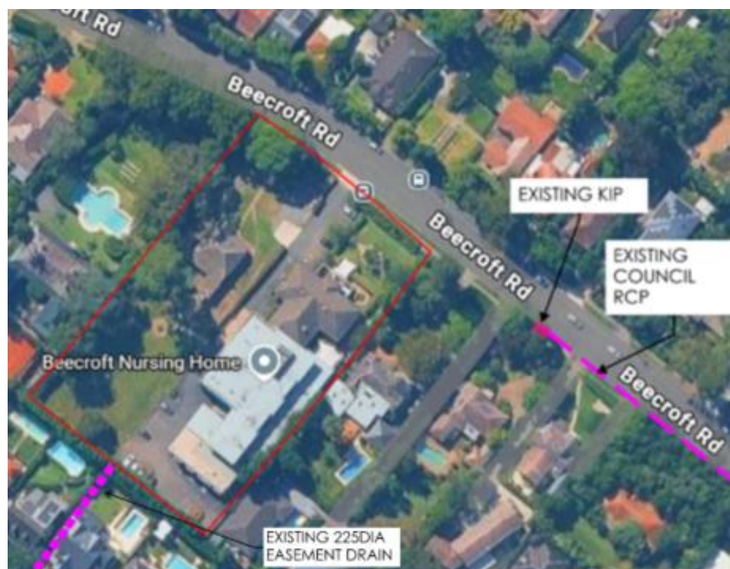
Figure 3 – Council stormwater drainage map
