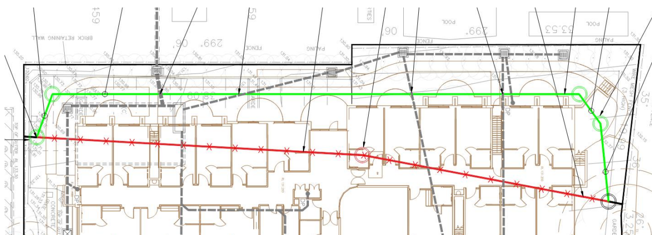
Figure 5 – Proposed sewer diversion
