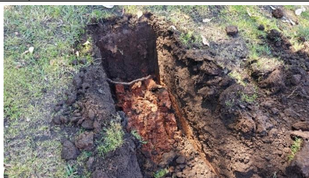
Image 4 - Typical soil profile (TP14)
