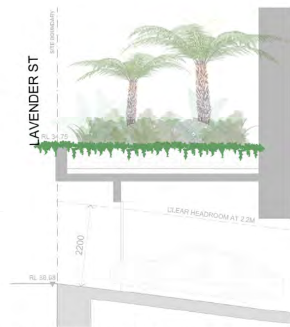
cc TYPICAL SECTION - PLANTER OVER DRIVEWAY
