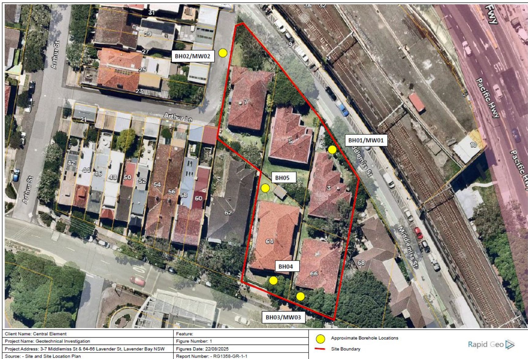
Figure 23 – Locations of the geotechnical testing locations
