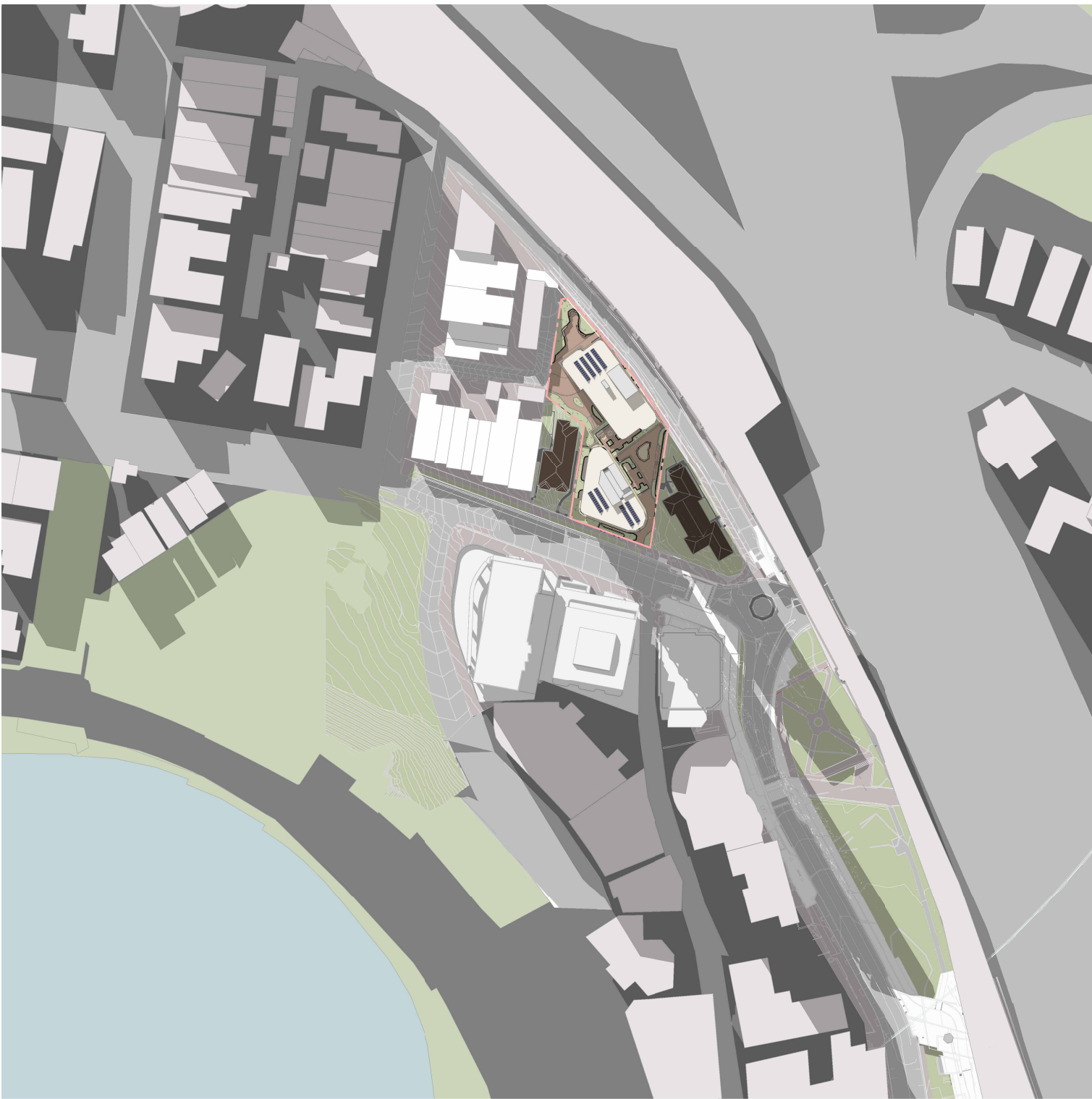
6 SHADOW PLAN - 02.00pm DA-1401 SCALE 1:2000
