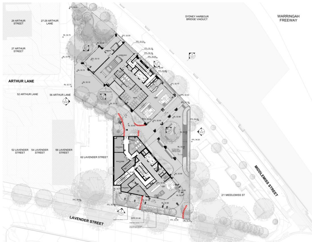
Image 6a: Recommended Wind Mitigation Measures – Ground Level
