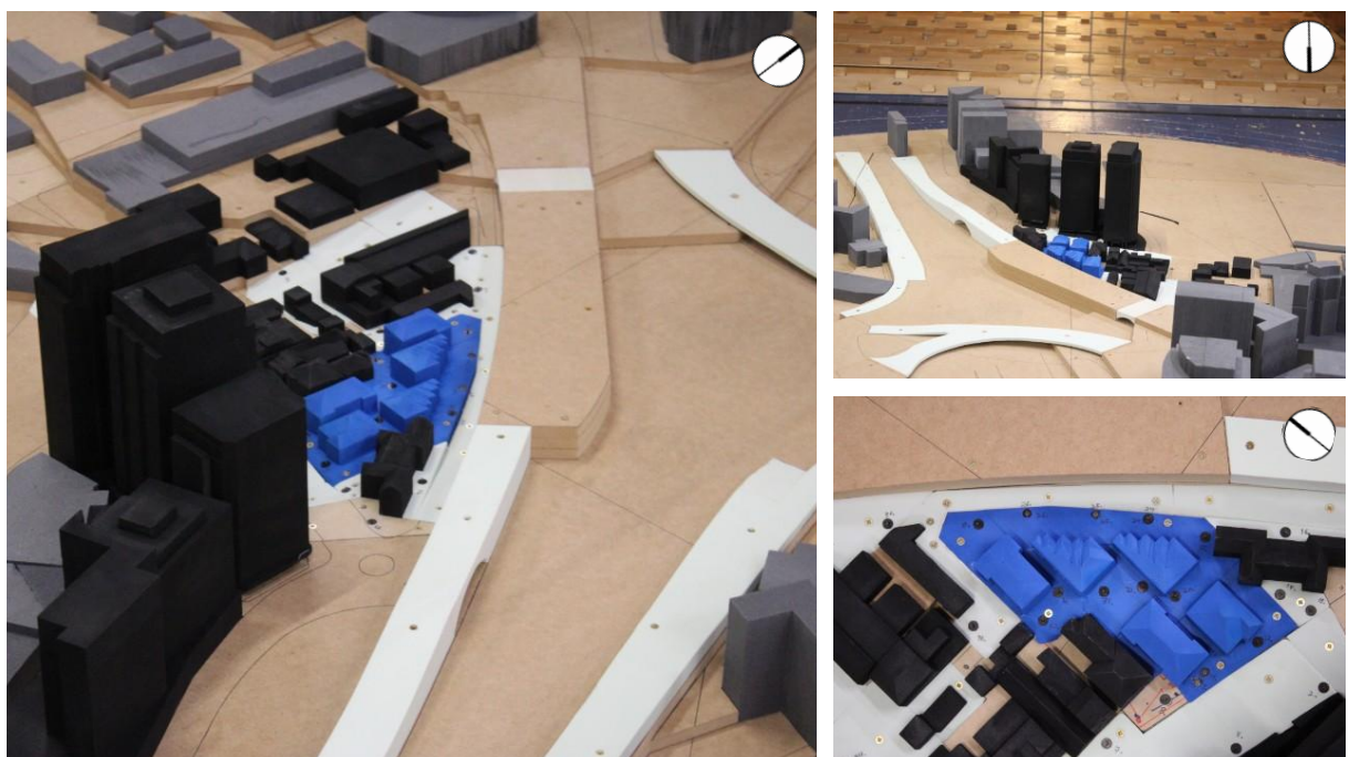
Image 2A: Wind Tunnel Study Model – Existing Configuration
