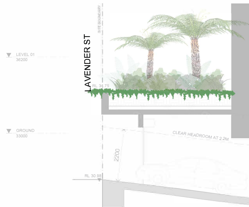
cc TYPICAL SECTION - PLANTER OVER DRIVEWAY
