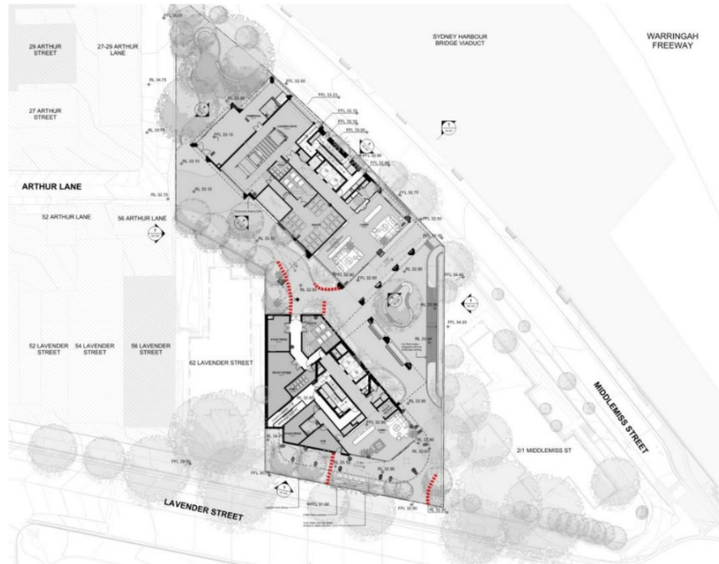
Image 6a: Recommended Wind Mitigation Measures - Ground Level
