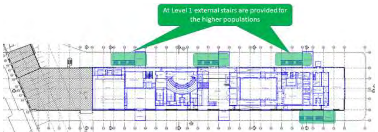
Figure 11: Pier 2/3 Level 1 egress
