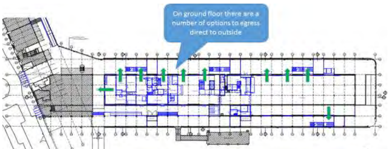
Figure 9: Pier 2/3 ground floor exit
