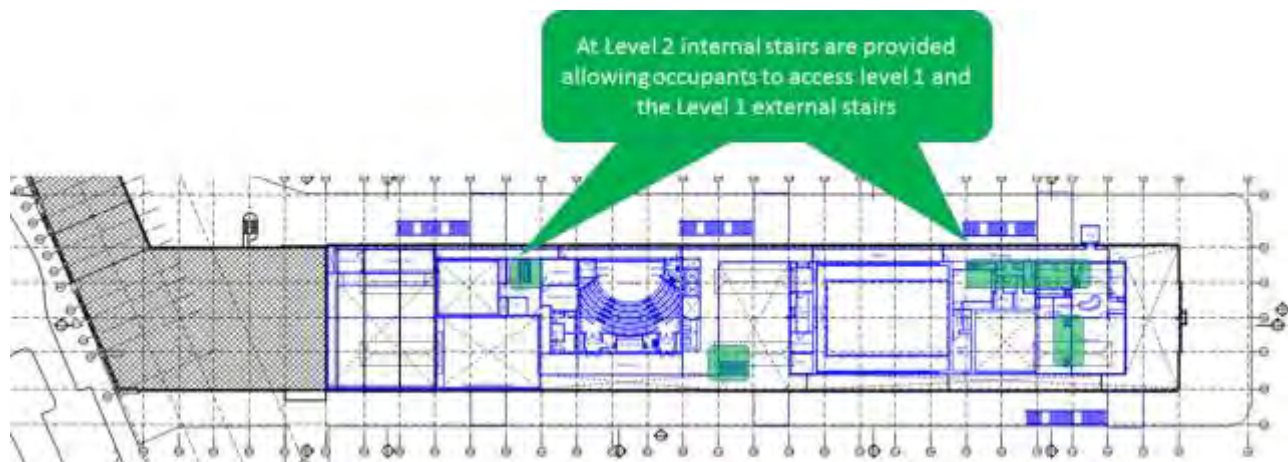
Figure 12: Pier 2/3 Level 2 egress
