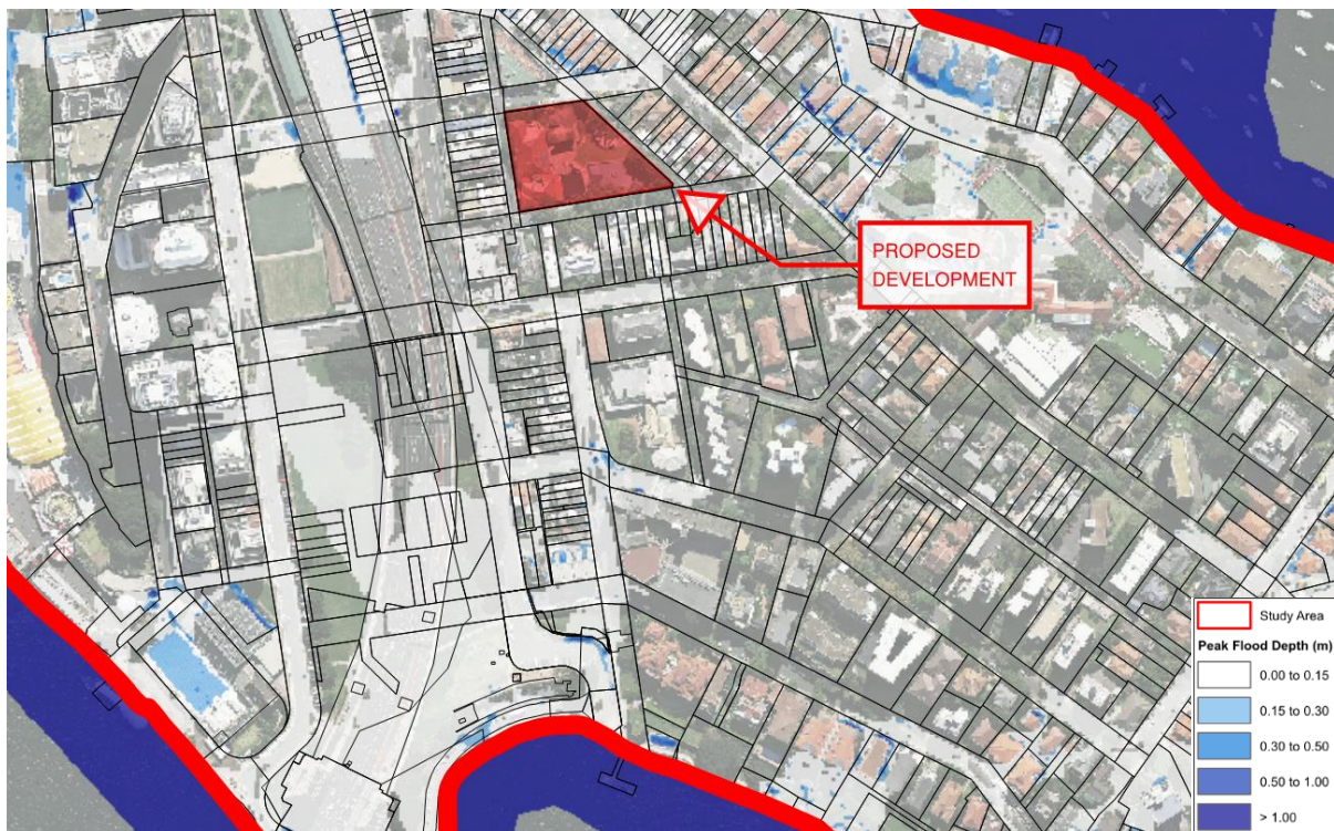
Figure 3: Peak Flood Depth and Flood Level Contours 1% AEP (Source: North Sydney LGA Flood Study WMA water – February 2017)
