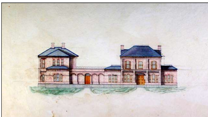
Figure 2.7 Undated, early elevation showing a scheme for two pavilions and attached single storey wings.
