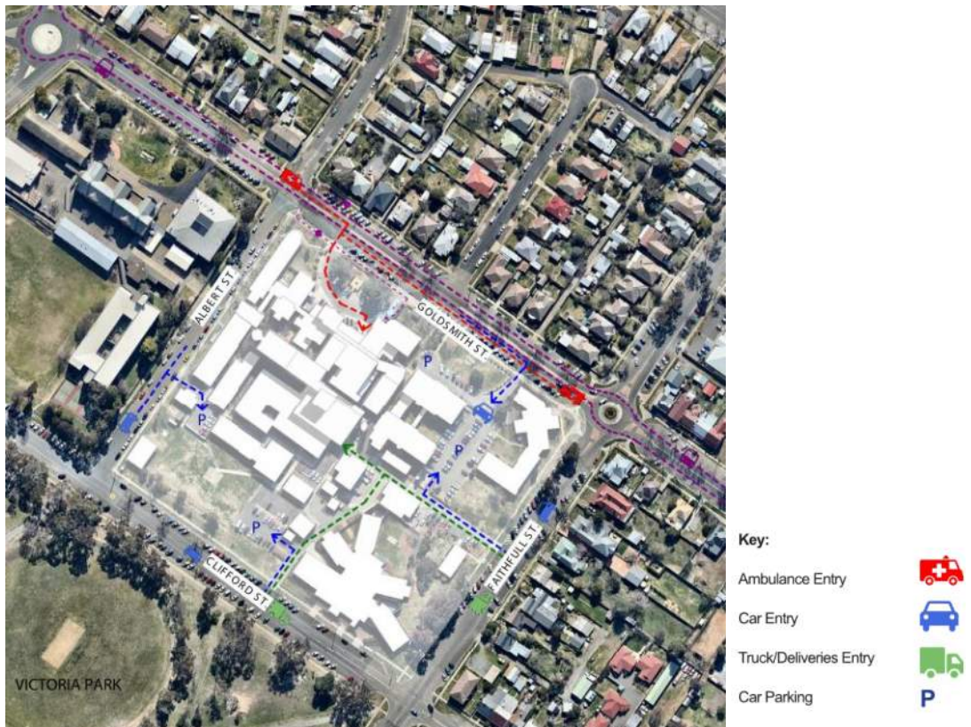
Figure 13: Site plan showing primary transport, ambulance, delivery and logistics, public transport and car parking access (Source: BLP)
