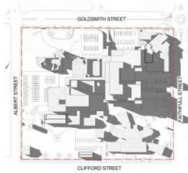
Figure 54: Winter solstice solar access diagrams extracted from Architectural Design Summary (Source: BLP).
