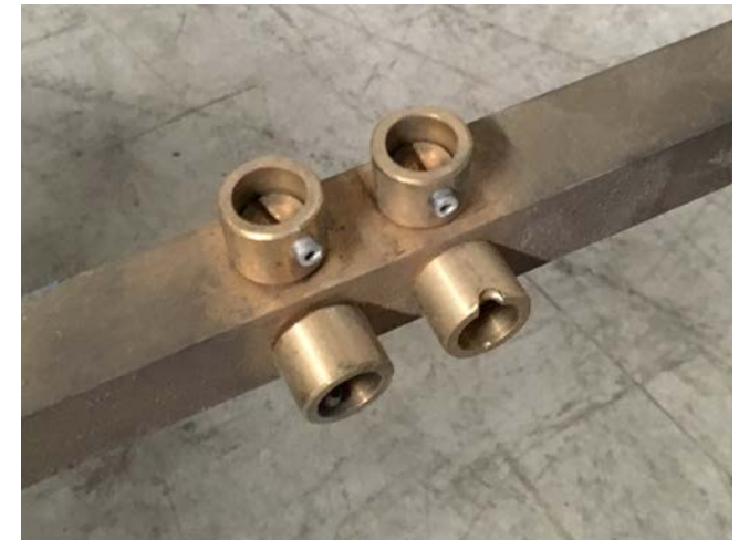
01 Sample of brazed joint.
