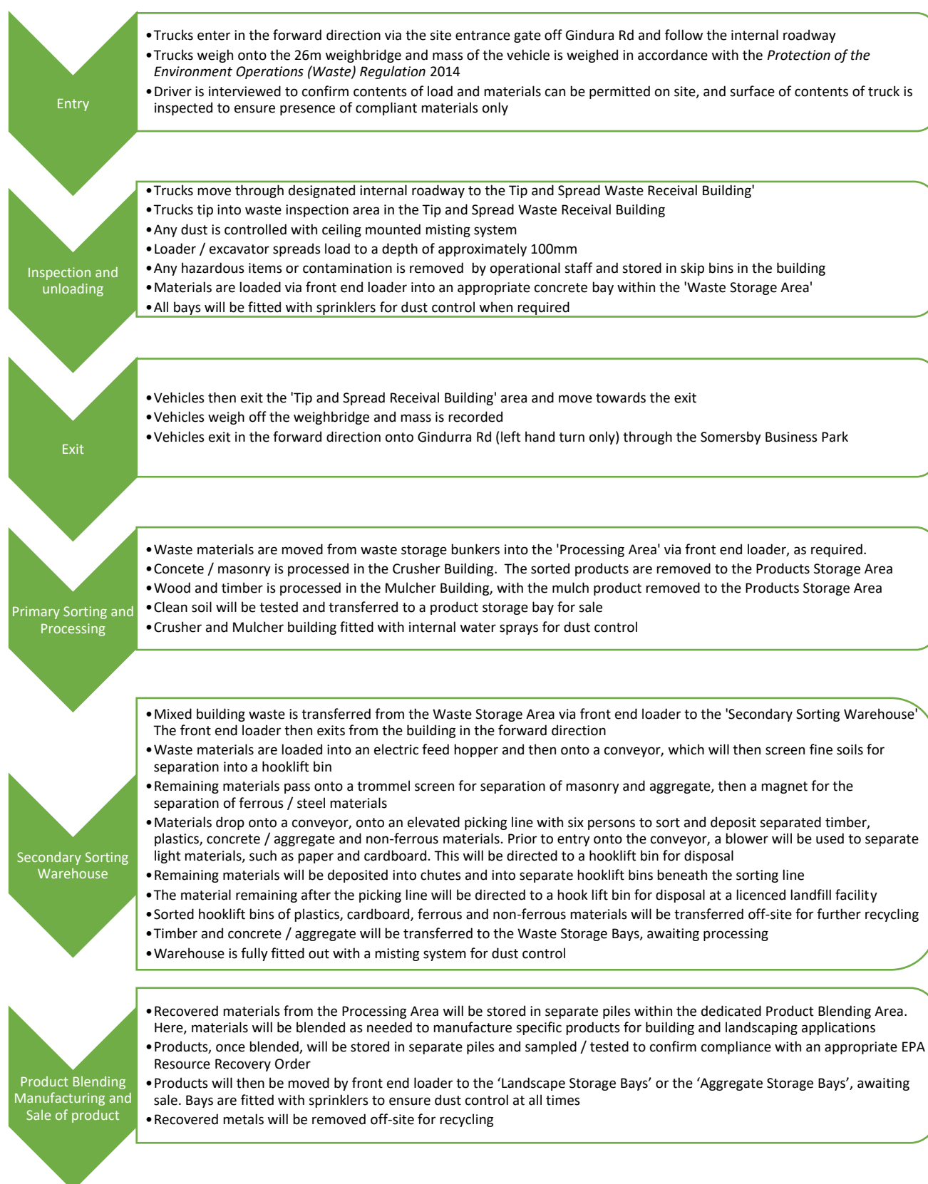
Figure E1. Process flow chart for recycling operations.
