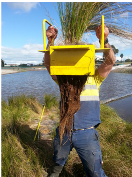
Figure 1. Specially fabricated removable planter boxes to assess root length.
