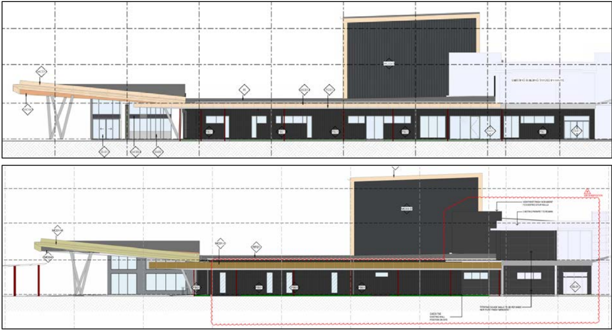
Figure 4 | Approved western elevation (Main Entry) (above) and proposed western elevation (Main Entry) (below) (Source: SSD 8647 Approved Plans and Applicant’s Modification Report)
