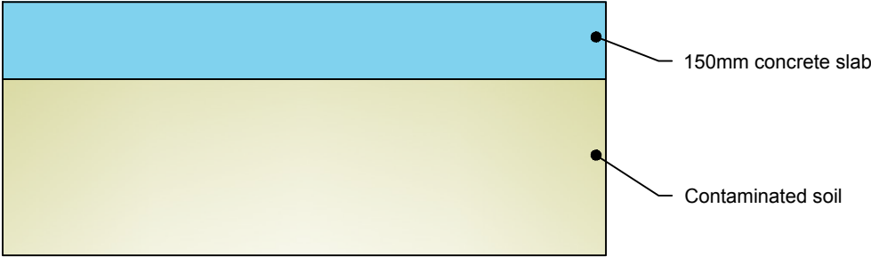
Cap No.1 - Existing Concrete
