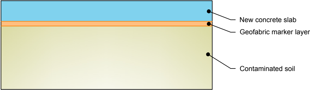
Cap No.2 - Concrete (As yet constructed)
