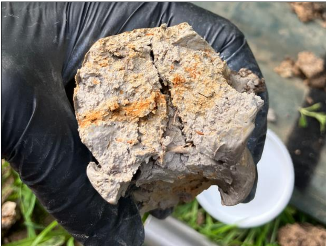
Site Photograph 2. View of representative inferred natural CLAY materials (0.6 – 1.5 m bgs) encountered across the site, as observed on 8 July 2025 within sampling location 'BH01'.
