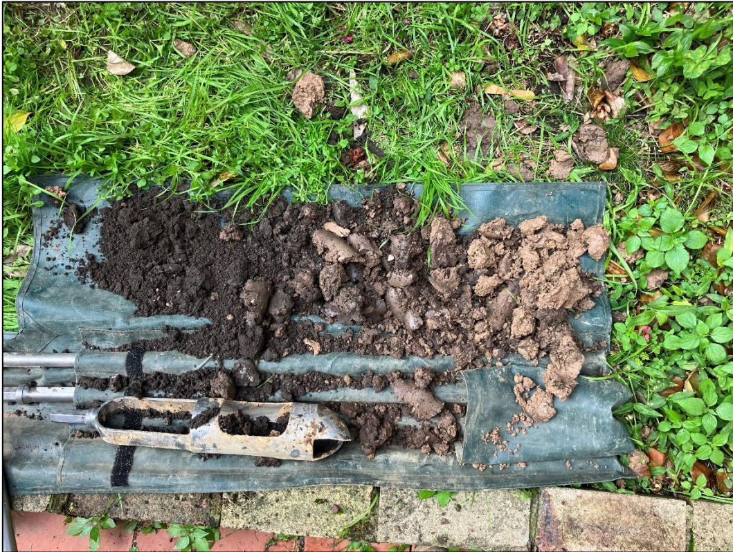
Site Photograph 1. Representative view of soil materials encountered across the site, as observed on 8 July 2025 within sampling location 'BH01'.
