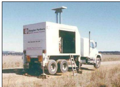
Figure 2: Purpose built CPT rig
