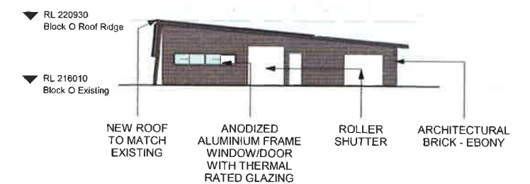
7 EAST ELEVATION - METALWORKS 1:200
