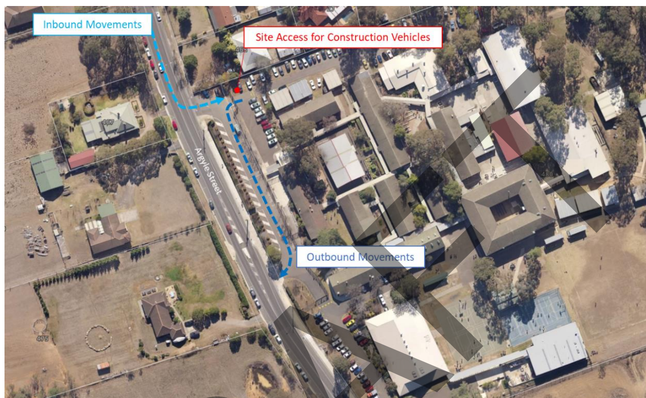
Figure 3-1: Construction Vehicle Movement Plan 1
