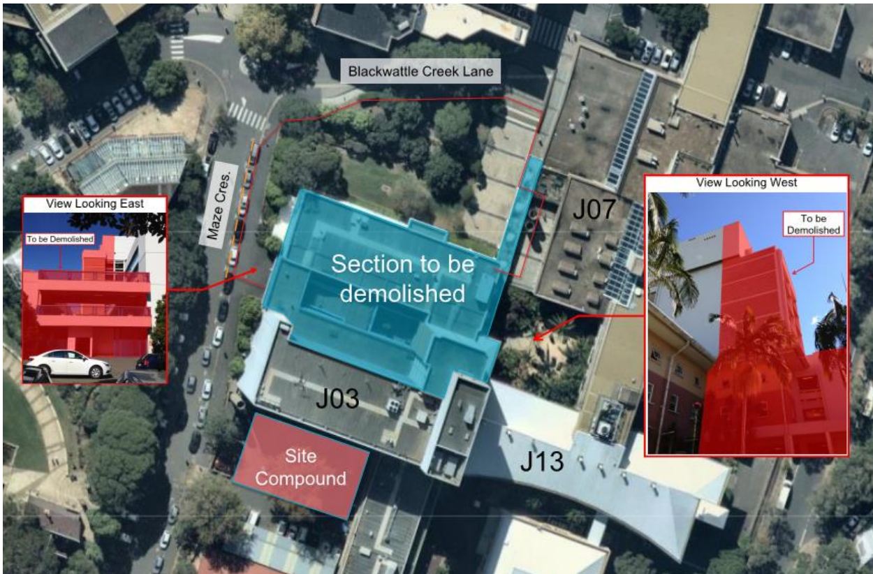
Figure 21: Demolition location plan
